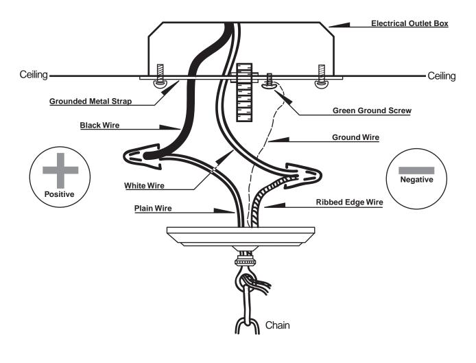
**NOTE:** *Connect Wires As Shown!* Installation must be performed by a qualified electrician. Studio Steel Warranty and Damage Claim VOID where wiring has been spliced, replaced, or compromised. This diagram is a representation only, and is not intended as a construction document.
